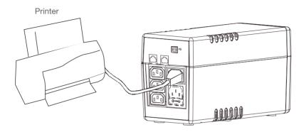
Note: DO NOT plug a laser printer, copier, space heater, vacuum or other large electrical device into the UPS. The power demands of these devices will overload and possibly damage the unit.
